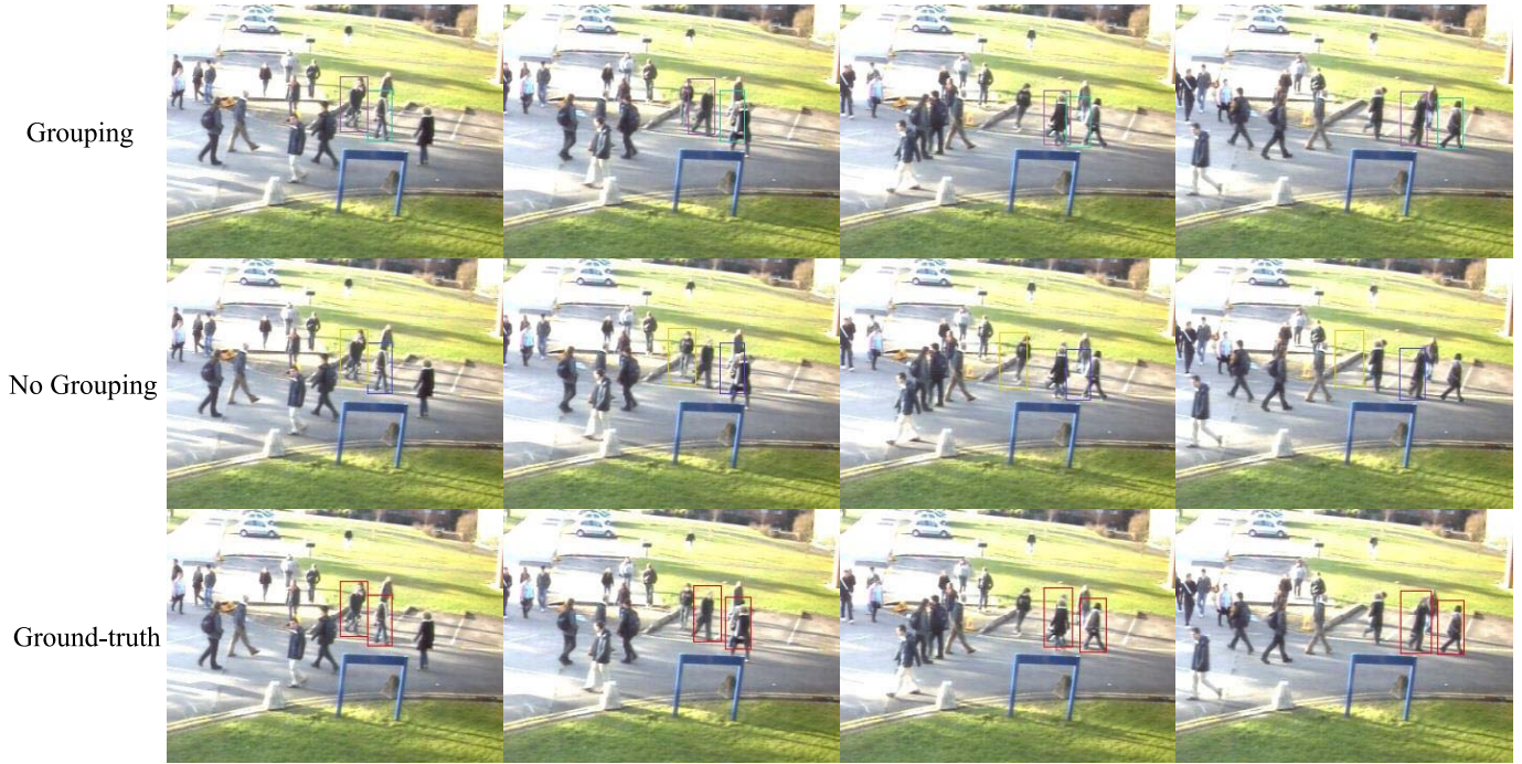
Fig. 4. Sample frames for tracking two pedestrians in a group using two different strategies. From the left column to the right column, four frames (#048, #053, #058, and #063) are shown. The top two rows show the tracking results with and without grouping, respectively. The last row contains the corresponding ground truth. Frames are enlarged and cropped for better illustration.
